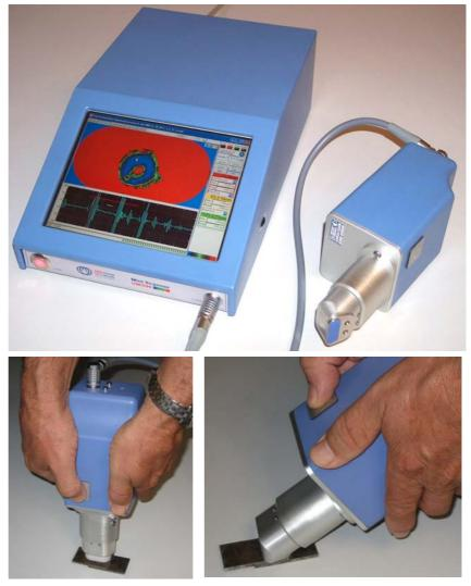
All data, including the complete A-scan information, can be stored on the hard disk. This is useful for evaluation purposes and after event setting control. With exchangeable scan-heads for perpendicular or angled scanning position the "Mini Scanner" can be used for a wide range of applications.
